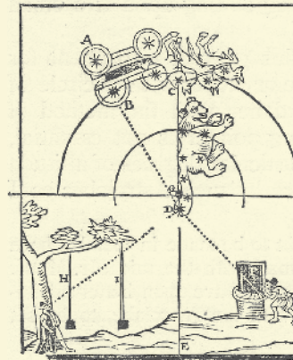
Below: Blagrave's method of drawing the meridian line in the night by the Pole Star. Art of Dyalling , 1609, p. 73
