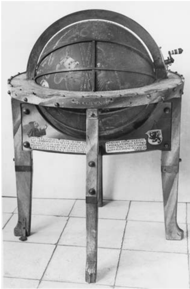
FIG. 6.11. CELESTIAL GLOBE FROM STÖFFLER'S WORKSHOP. The globe was made in 1493 in the workshop of Johannes Stöffler, an astronomer and instrumentmaker who was professor of mathematics at the University of Tübingen. The metal grid surrounding the globe is for astrological purposes such as making horoscopes. Size of the original: diameter 49 cm; height 107 cm. Photograph courtesy of the Germanisches Nationalmuseum, Nuremberg (inv. no. WI 1261).
